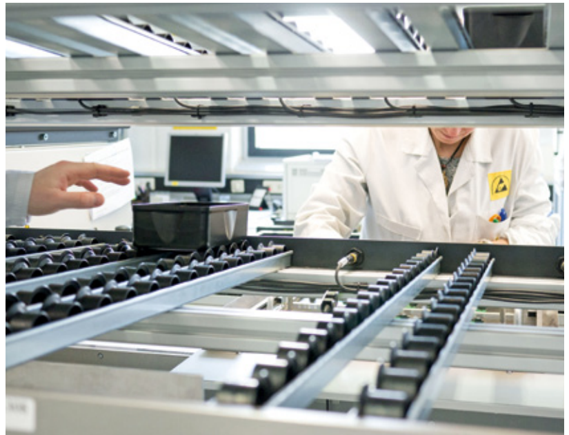
Both shelving systems can be filled with new components from the back without interrupting the production process
