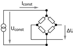
The bridge voltage ( $U_{const}$ ) is the product of the constant current ( $I_{const}$ ) and the equivalent resistance of the bridge (parallel/series arrangement of the four individual resistors). For example, if a constant current source of 20 mA is supplying the circuit, there will be a bridge voltage of 15 V with a bridge resistance of 750  $\Omega$ .
