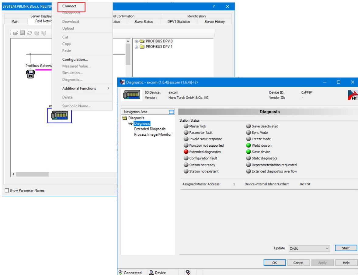
Fig. 23: Standard PROFIBUS diagnostics (listed according to significance)
