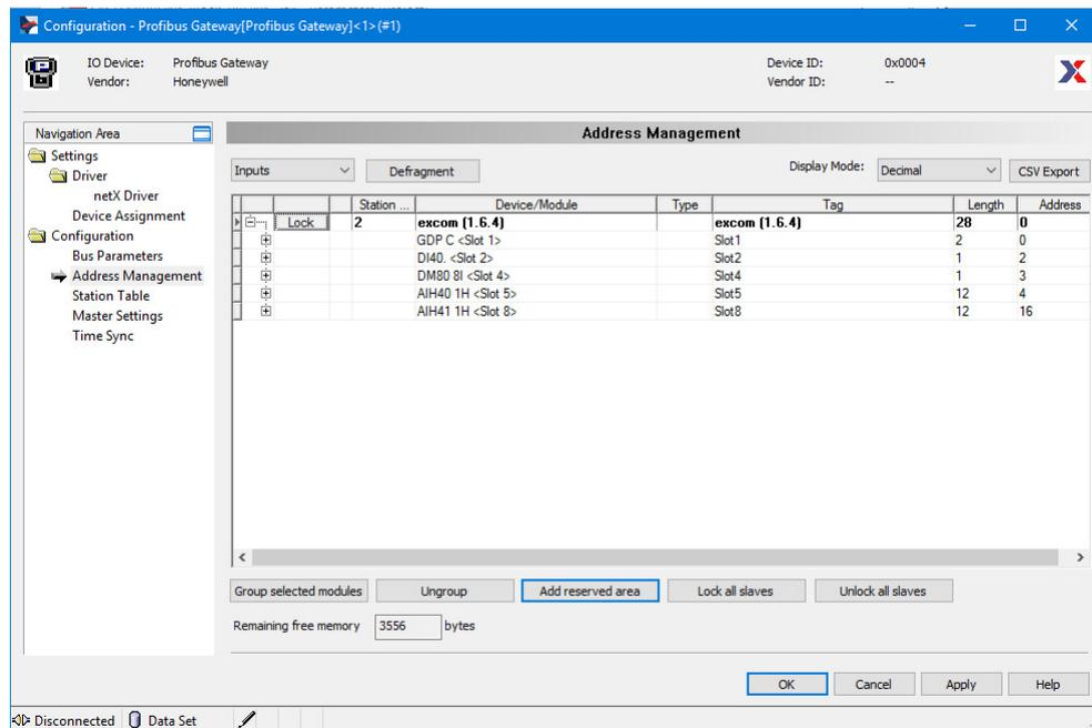
Fig. 36: Expanding the memory for excom® modules
