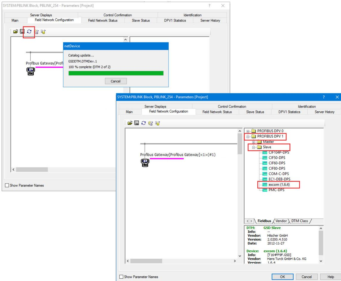
Fig. 3: Installing GSD – Selecting excom®
