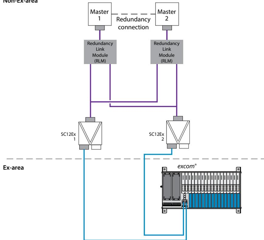
Fig. 28: Redundant setup with 2 masters and 2 segment couplers (example)
