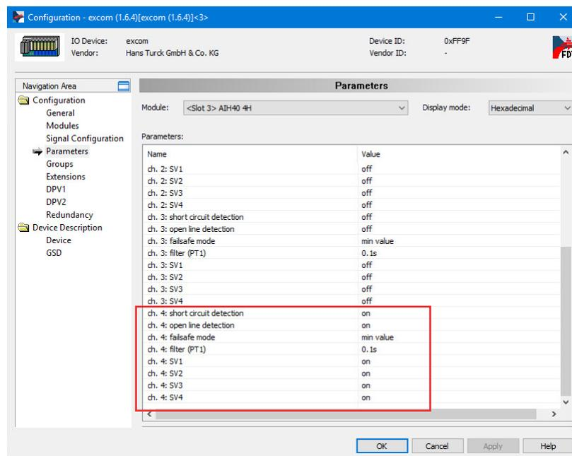
Fig. 39: Setting HART® communication for AIH40-4H with level sensor on channel 4
