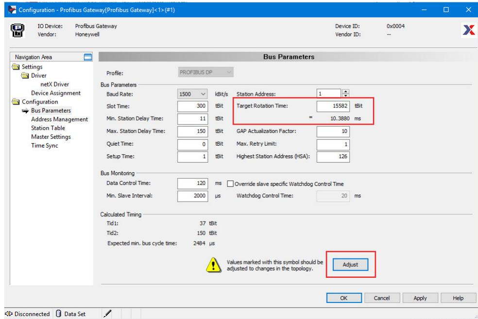
Fig. 37: Adjusting the bus cycle time
