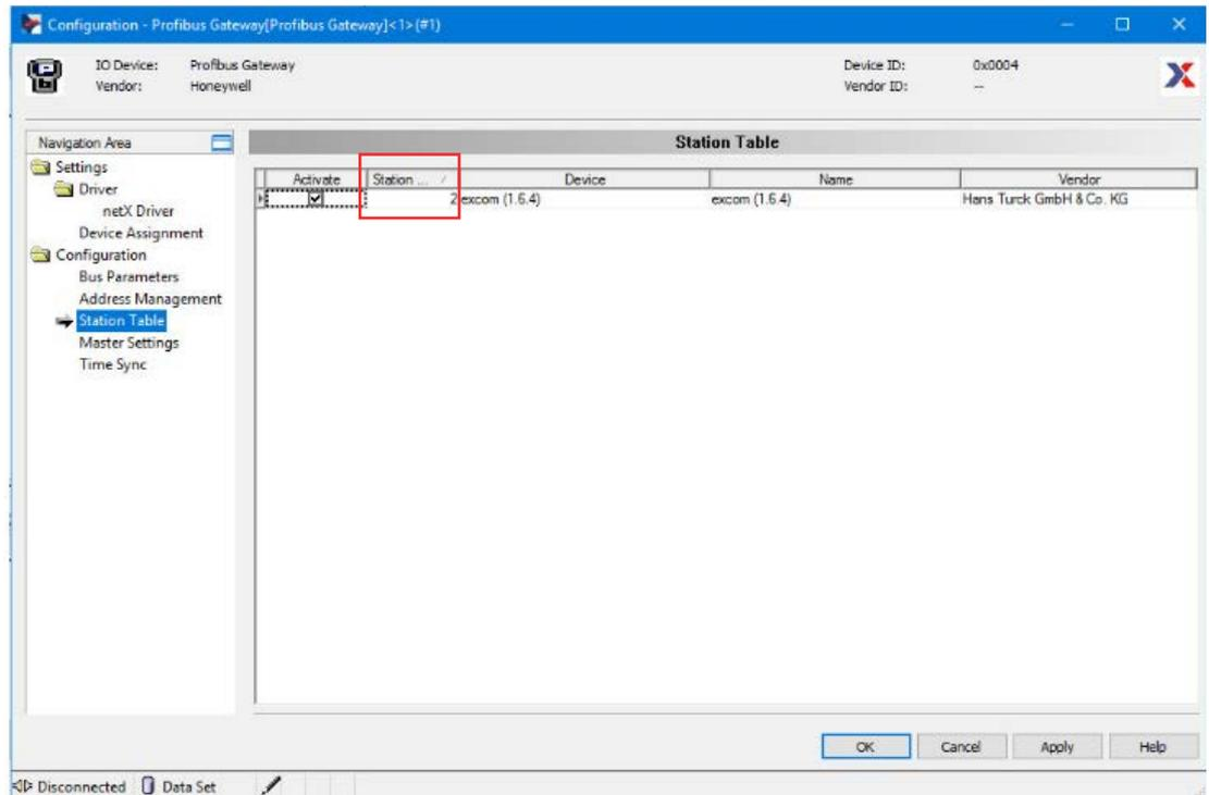
Fig. 9: Entering the slave address (example: 2)
