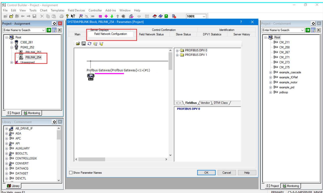
Fig. 2: Installing GSD – Selecting a PROFIBUS link
