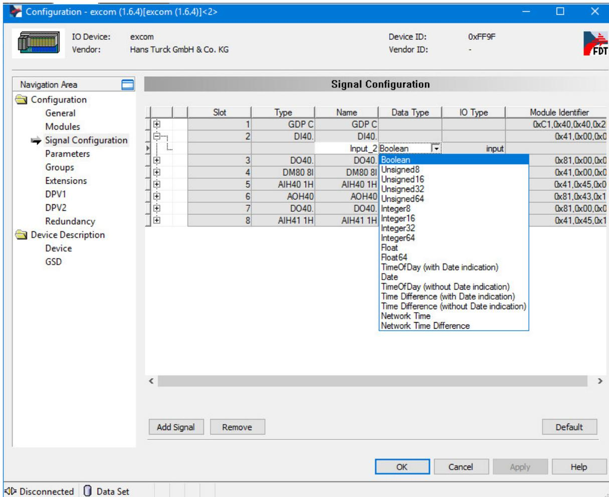
Fig. 13: Configuring I/O data – Changing the name and data type of a module
