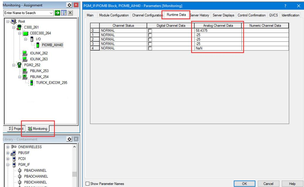
Fig. 21: Example: Process data for AIH40, 1st channel actively supplied
