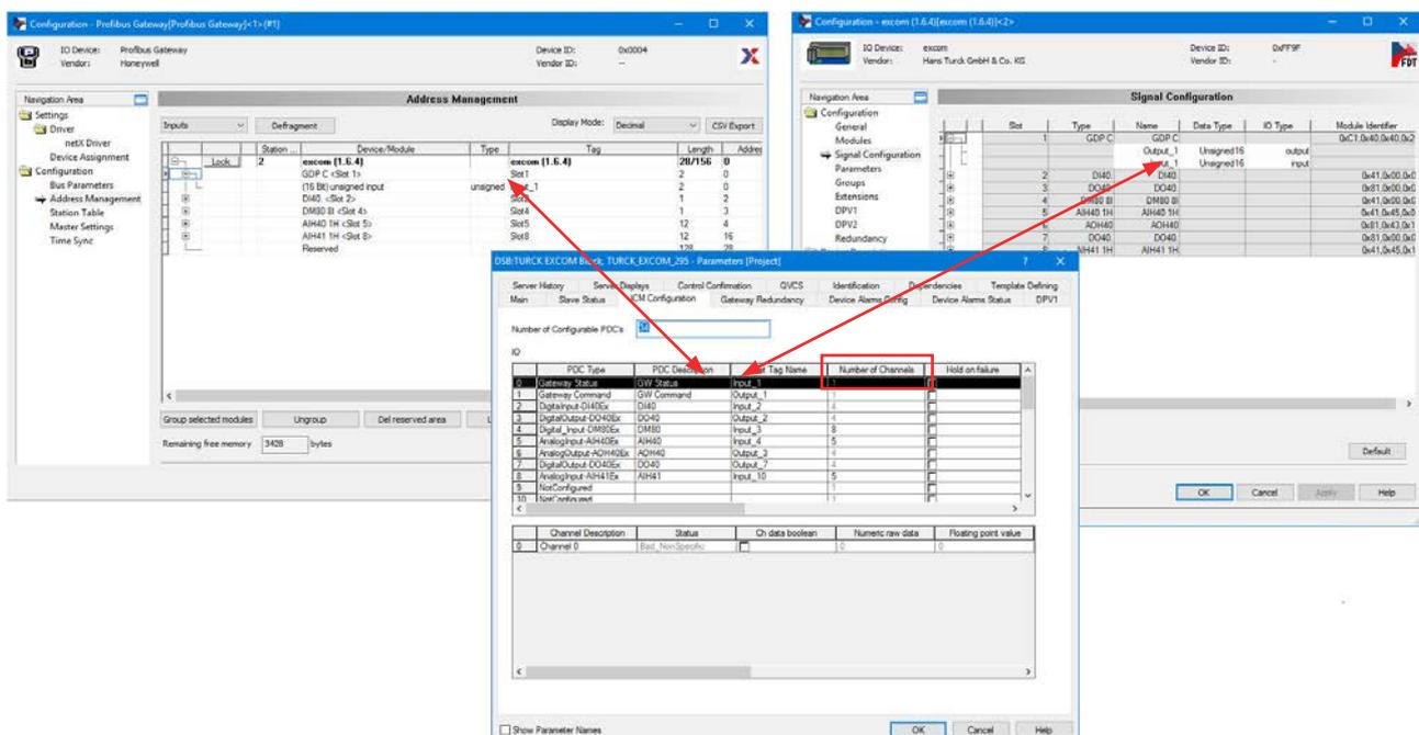
Fig. 15: Configuring I/O data – Creating a PDC
