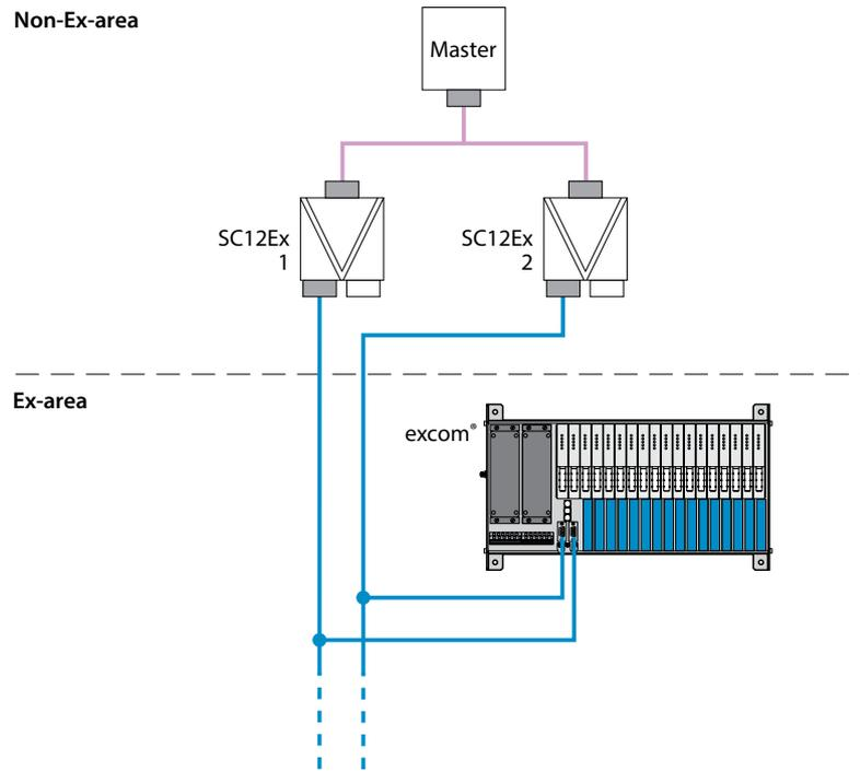
Fig. 27: Redundant setup with one master and 2 segment couplers (example)
