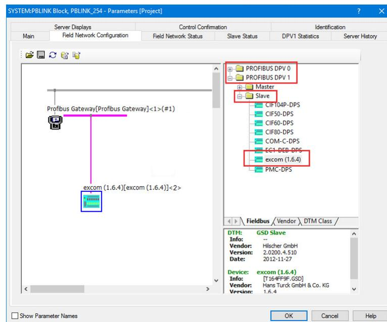
Fig. 4: Creating a PROFIBUS slave (example: PROFIBUS DPV 1)
