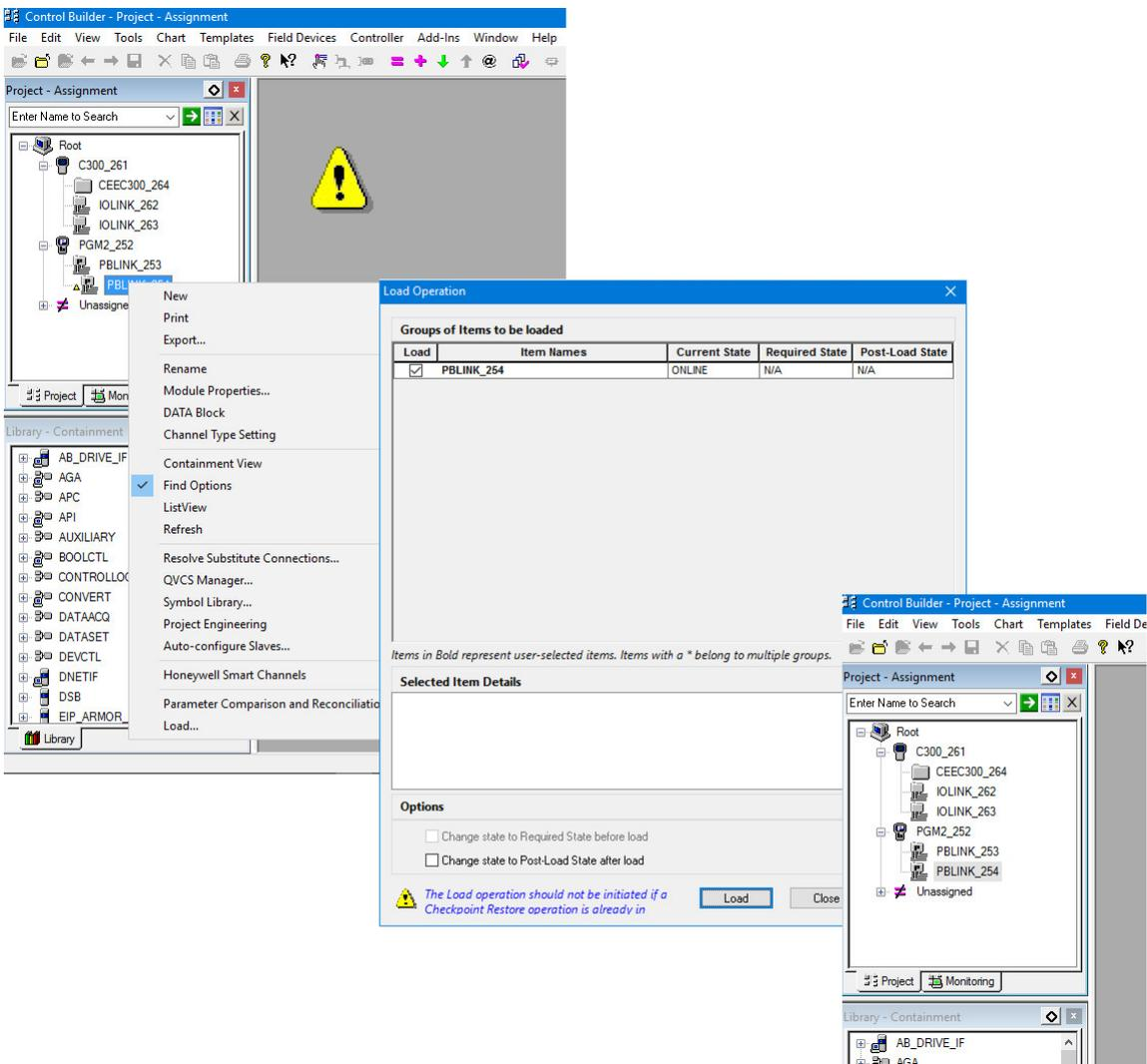
Fig. 12: Transferring parameters to the controller
