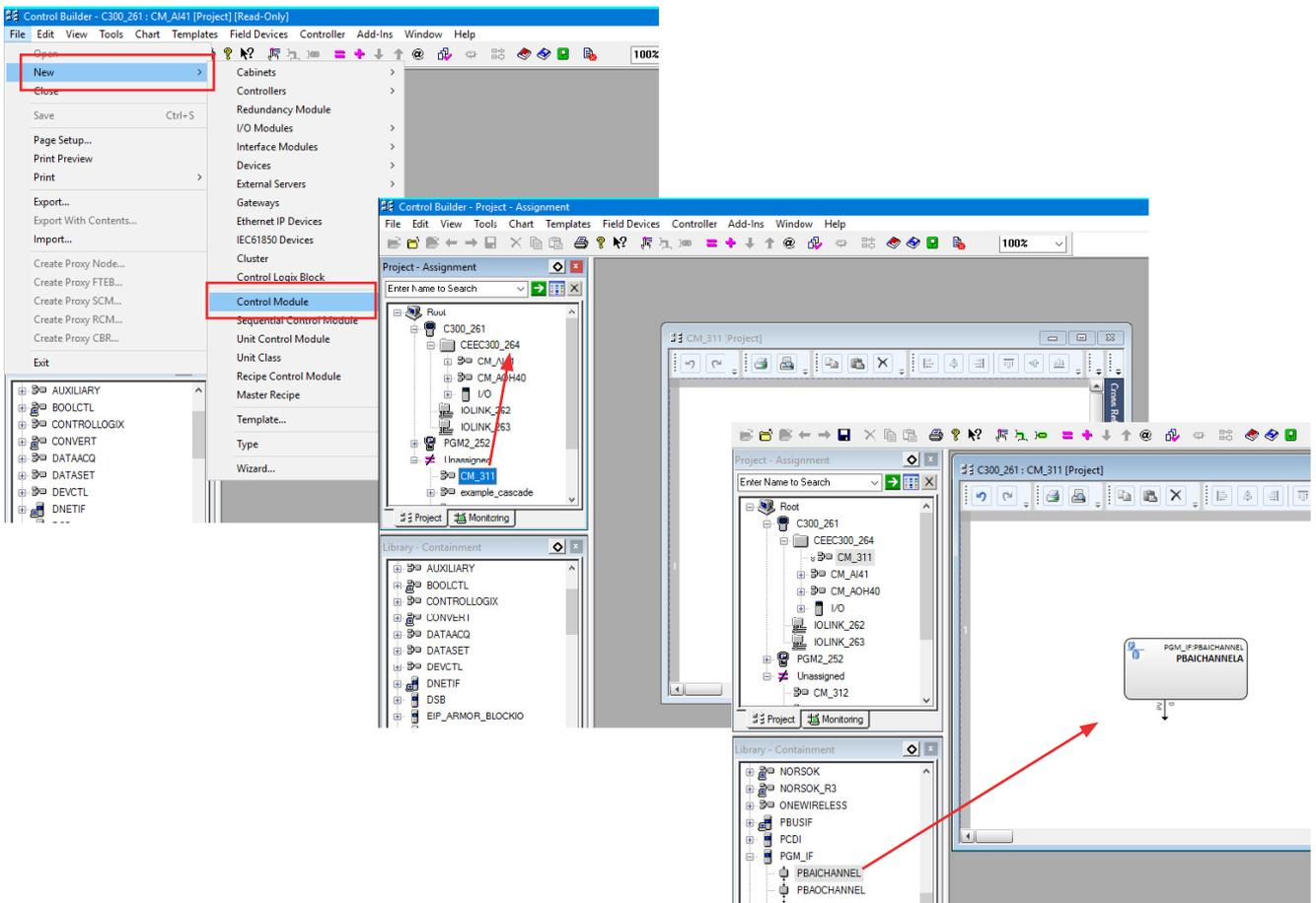
Fig. 18: Creating a PROFIBUS channel block (example: PBAICHANNEL – PROFIBUS analog input channel)
