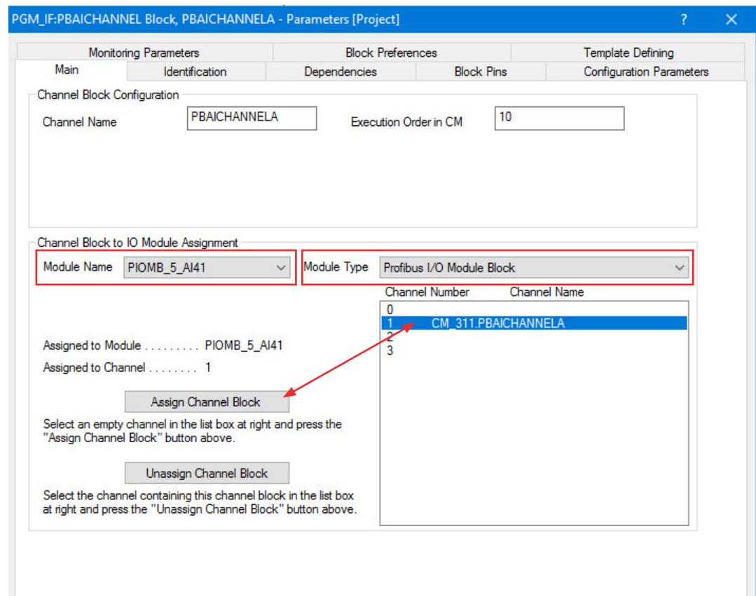
Fig. 19: Assigning a PROFIBUS channel
