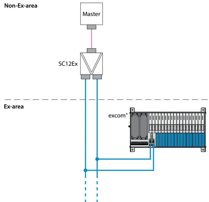
Fig. 26: Redundant setup with one master and one segment coupler (example)
