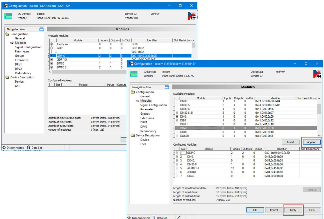
Fig. 6: Configuring an excom® station as a slave
