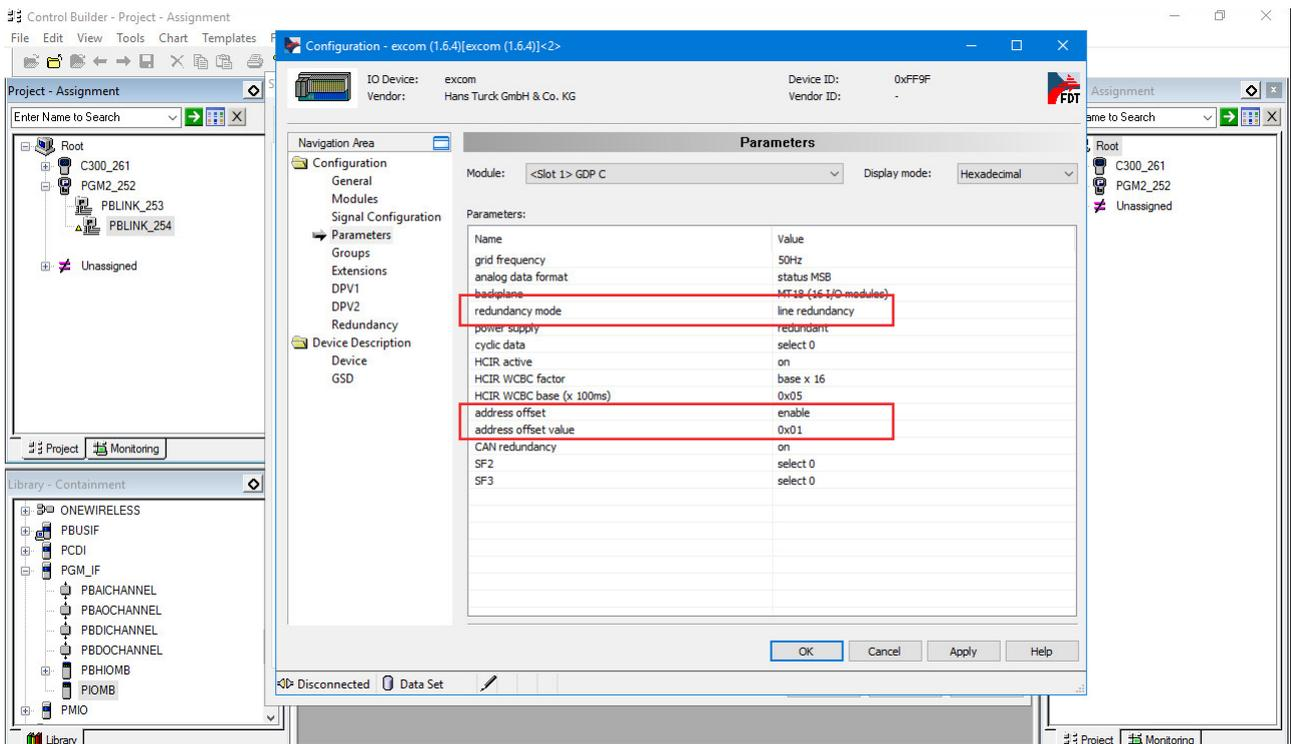
Fig. 29: Configuring and parameterizing redundancy
