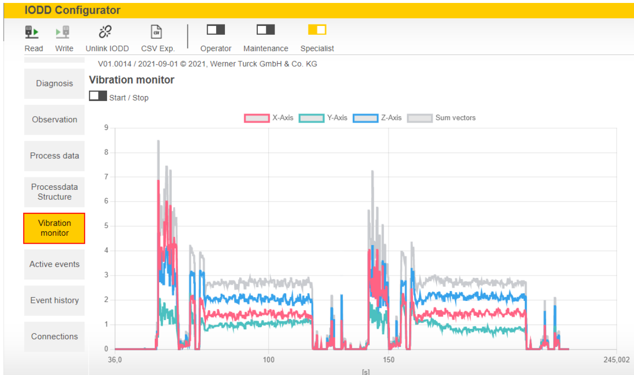
Fig. 11: Turck Vibration Monitor – overview
