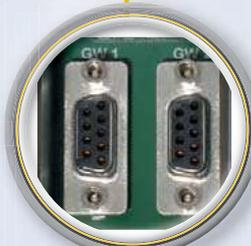
Connection of the higher-level PROFIBUS-DP fieldbus
