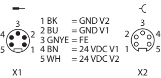
fig. 17: Pin assignment power supply connectors
