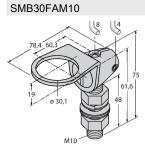
Mounting bracket, stainless steel, for M10 x 1.5 thread, thread length 30  $\,$
