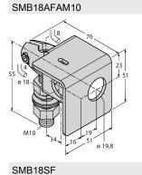
Mounting bracket, material VA 1.4401, for M10 x 1.5 thread, thread length 18 mm
