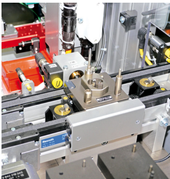
The reader reads the tag on the workpiece carrier in order to identify the individual components
