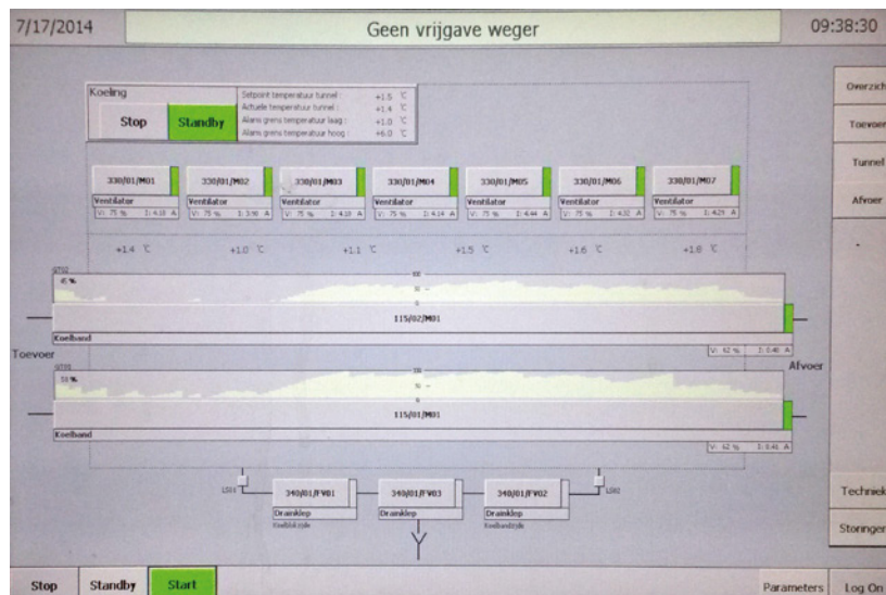
The two belts with the potatoes (in white) are visualized on the operator panel of the 57 controller
