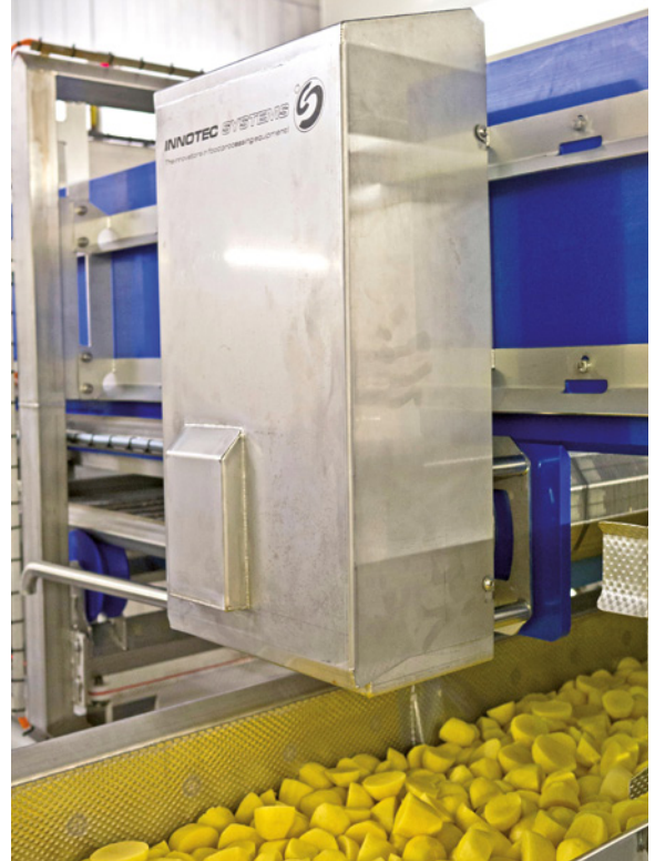
Double protection: The stainless steel guard covers the entire motor together with the encoder during operation
