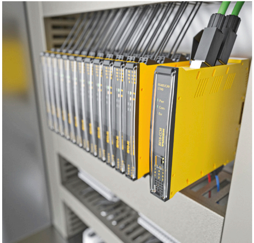
Turck's IM18-CCM cabinet guard transfers measured values via Ethernet to IT networks and can even preprocess them remotely beforehand
