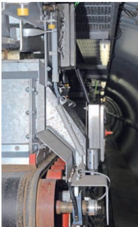
Rotary position sensors (bottom right) and inductive threaded pipe sensors (top left) continuously monitor the transport system and allow automated mixing processes
