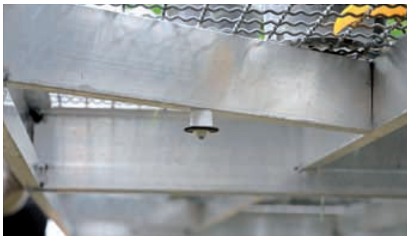
Precise identification: Each container carries a RFID tag on its bottom side
