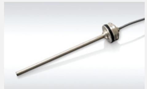
Turck is adding the robust LTE sensor for direct integration in hydraulic cylinders to its portfolio of linear position sensors. The magnetostrictive sensor can withstand shocks of up to 100 g and the vibrations that typically occur with agricultural and forestry machinery. The device is also insensitive to external influences, so that the LTE is even suitable for use in the hydraulic cylinders of construction machinery in extremely severe environments.
