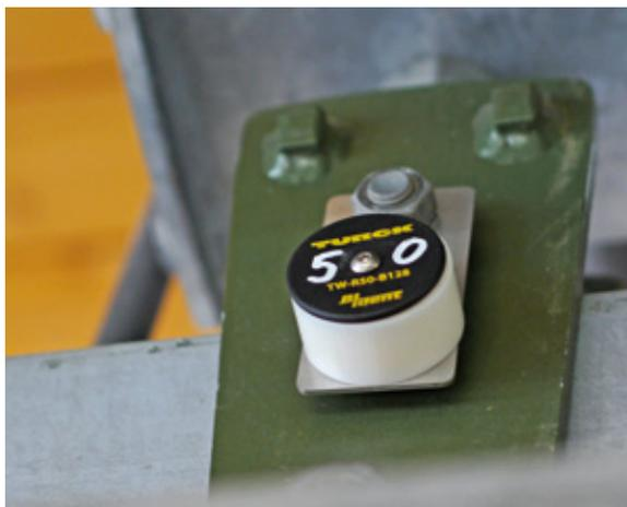
The Wie-Flyer track in Brotterode is equipped with RFID tags
